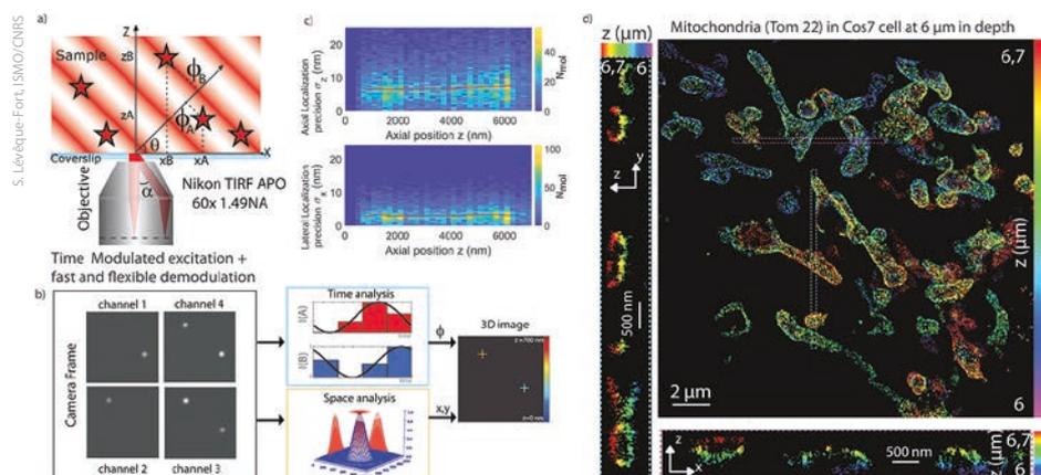
a) Introduction of a tilted, structured illumination pattern to encode axial information; b) modulated fluorescence is sampled at ~kHz on four sub-arrays on the camera to retrieve the phase; c) lateral and axial precision within the first 7  $\mu\text{m}$ ; d) 3D imaging of mitochondria in COS7 in dSTORM (Alexa Fluor 647)
