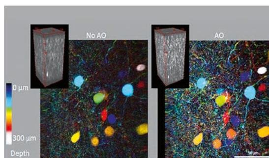
AO-TPFM for closed-loop correction in fixed brain slices. 2D maximal intensity projection of a stack of images in cortical brain slices of GAD-GFP mice without (left) and with (right) AO correction. Cell depths are colour-coded. Inserts: original Zstacks (S. Imperato, ESPCI and L. Bourdieu, IBENS)
