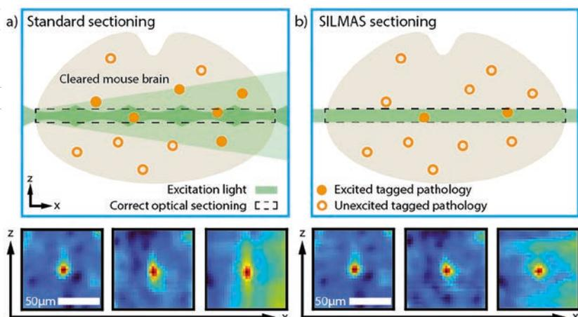
Comparison between standard sectioning in a) and SILMAS sectioning in b). Below are examples of fluorescent pathology at different penetration depths in cleared tissue. In a) the z-resolution is deteriorating with depth, while in b) the z-resolution is uniform throughout.
