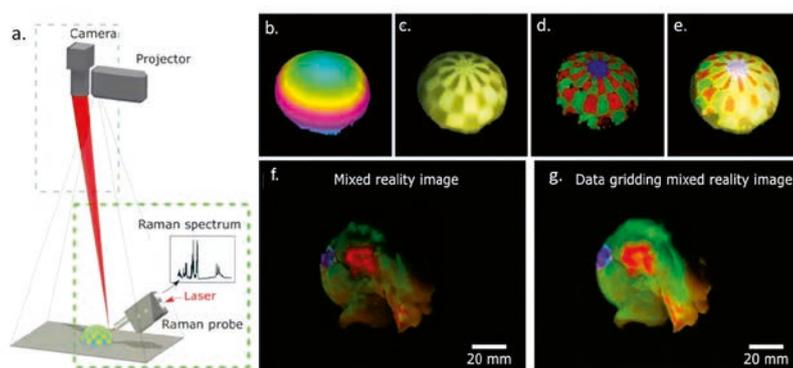
a. Raman-based system for the acquisition of MVR images
