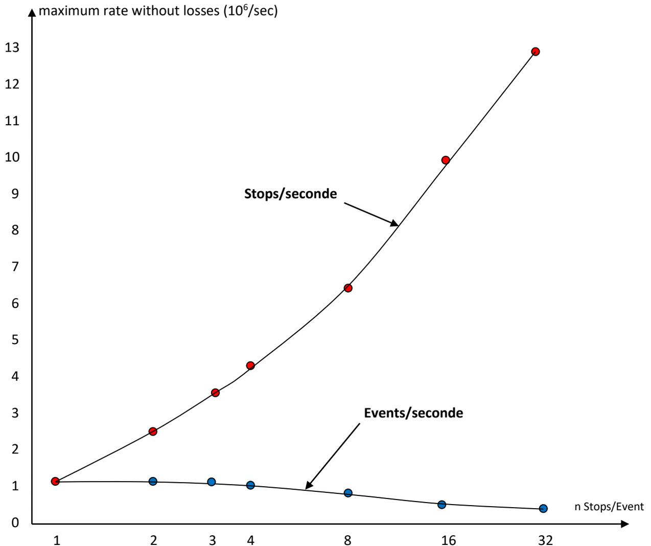
These maximum rates without losses are limited neither by the PCI Bus nor by the bridge to access it but by some compromises done in the FPGA of TDC-V4. Some amelioration is possible if necessary.
