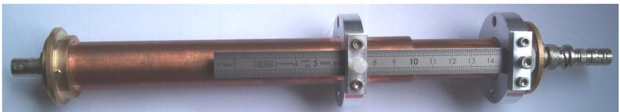
continuously variable length coaxial line
