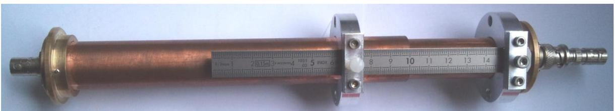
continuously variable length coaxial line
