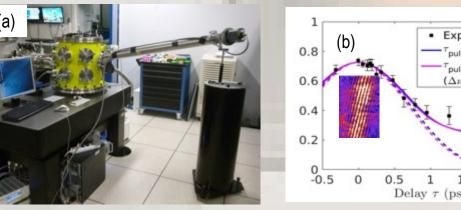
The partial temporal coherence of ultrashort plasma-based XUV lasers induces the formation of a pedestal in the shot-averaged autocorrelation signal (Fig. b) measured with the wavefront-division interferometer (Fig. a).
