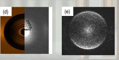
Photoelectron spectra obtained with (Fig. d) the plasma-mirror HH source @UHI100 (CEA Saclay), and with (Fig. e) the plasma-based XUV laser @LASERIX (Orsay), using the VMI spectrometer (Fig. c)
