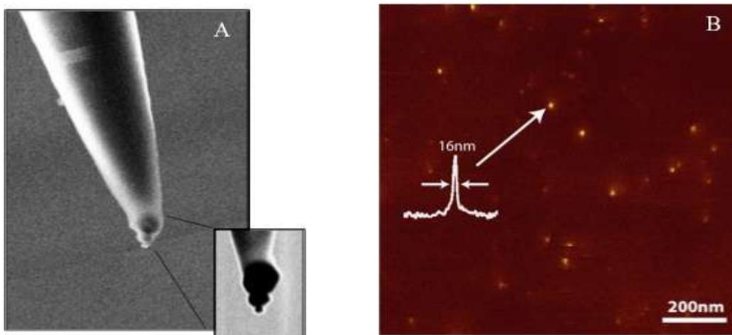
Fig. 1: (A) Electron micrograph of a self-similar trimer antenna comprised of three gold nanoparticles. (B) Fluorescence map of single molecules made using such an antenna showing sub-20 nm resolution
